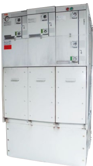
From IAC-test without arc suppressor
